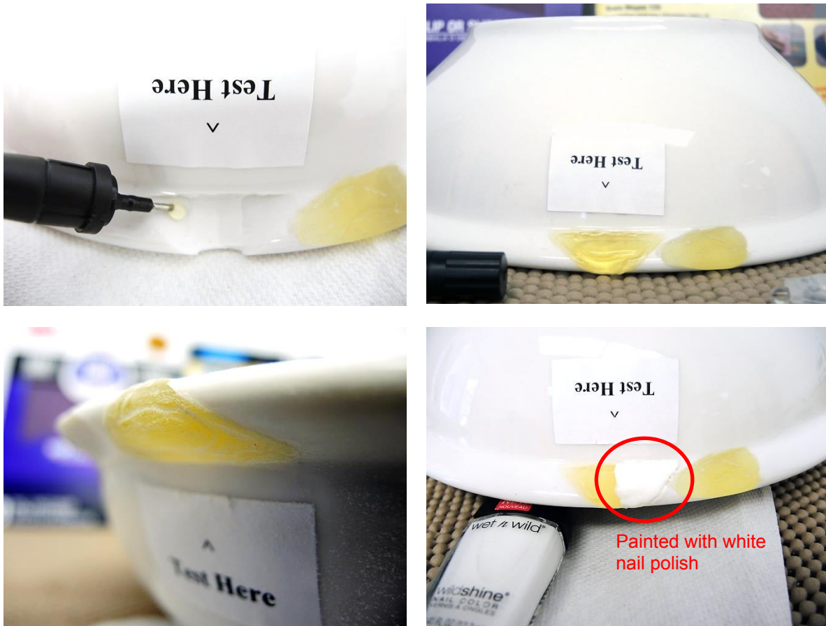
Figure 17: Bond to ceramic test. Brand was observed to be easy to use to fill-in the missing chip, and was then sanded for finishing, and painted with white nail polish.
