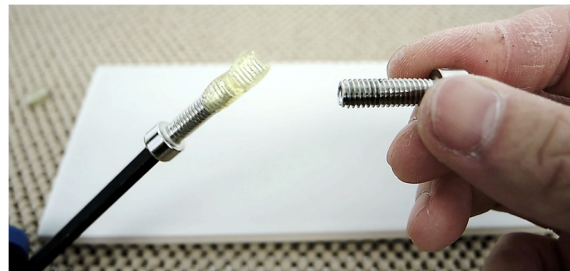
Figure 5: Confirming two screws can be unthreaded from the cured liquid.
