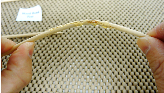
Figure 16: Third bond to wood test (a fixed wooden stick, bent from close edge).
