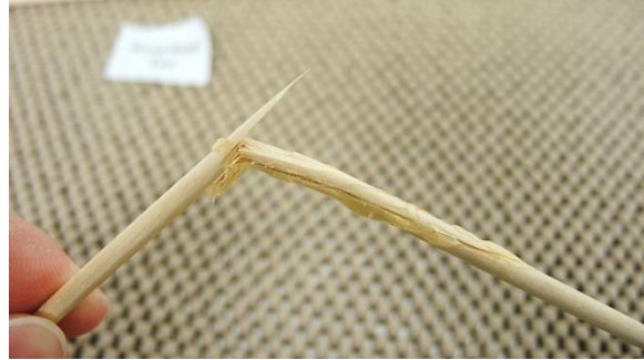
Figure 16: Third bond to wood test (a fixed wooden stick, bent from close edge).
