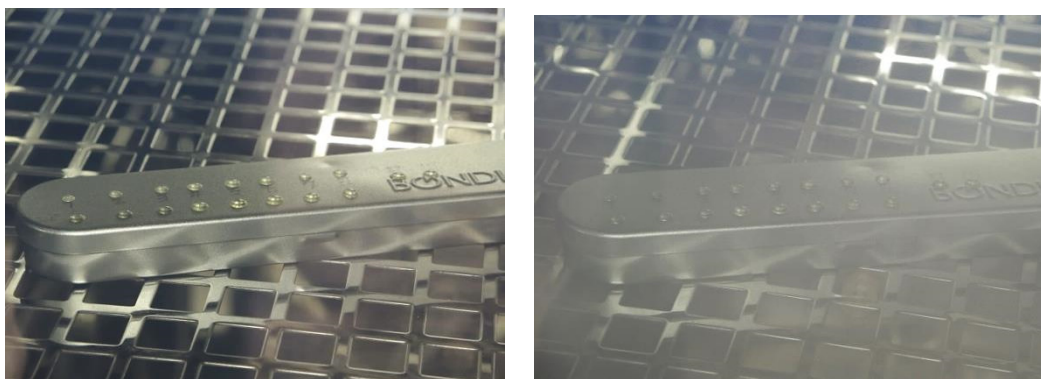
Figure 2: Ten cured liquid drops were subjected to -40°C (left) and +150°C (right).
