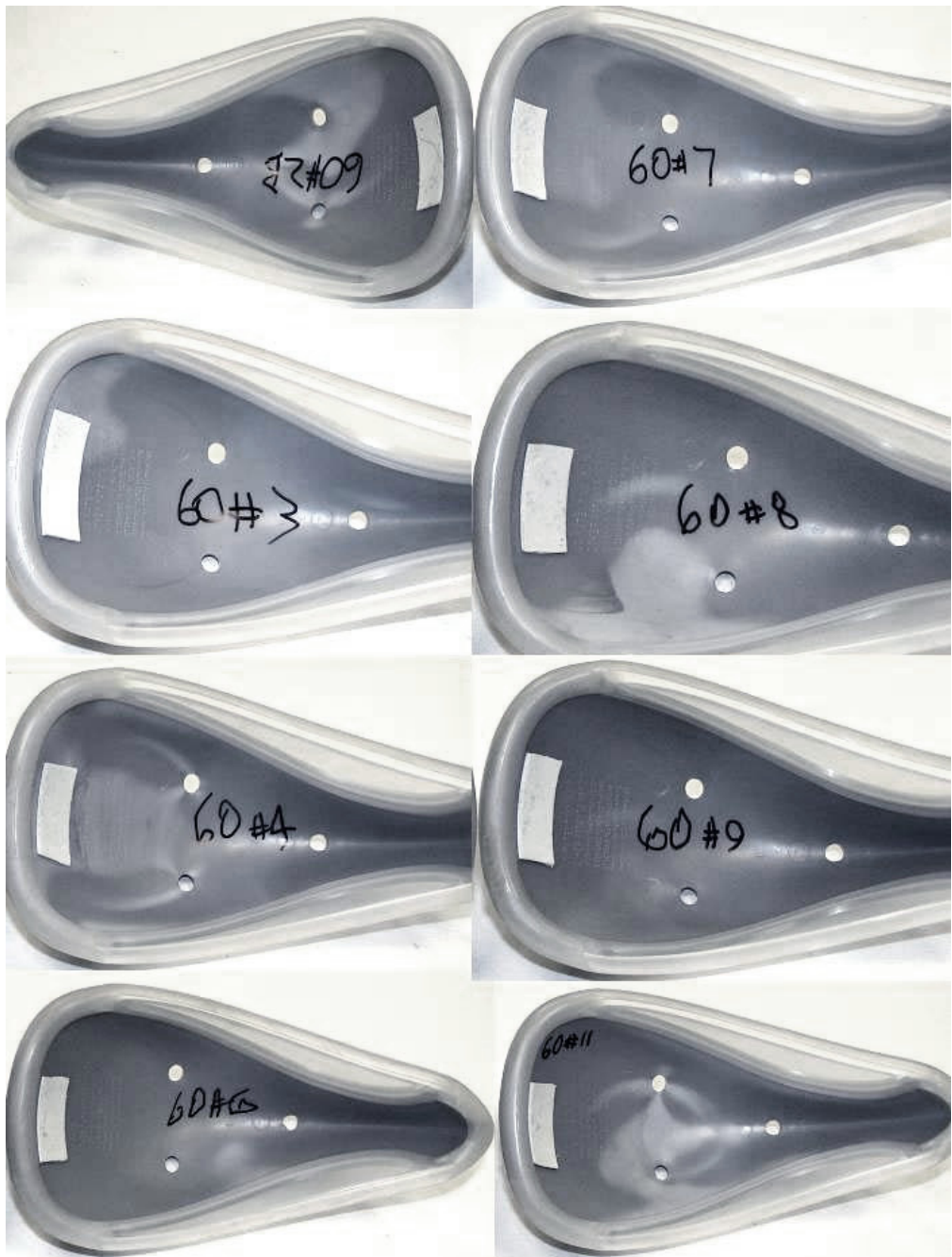
Impact stress marks on Brand - 3 cups struck at 60 mph
