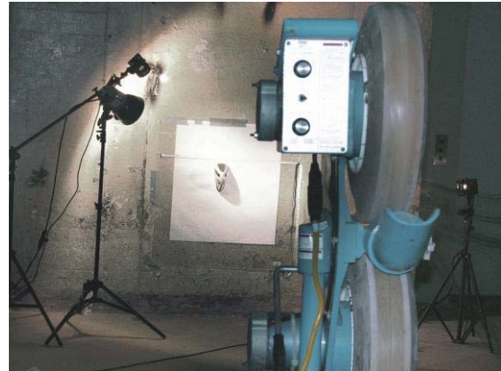
Looking downrange from behind the Jugs pitching machine. A third high-intensity lamp to the right side of the target is barely noticeable in this photo.
